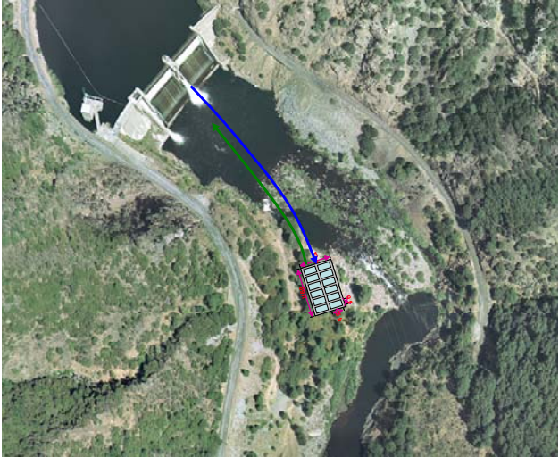
Figure 1a. Plan view of chiller location on Rock Creek Reach; Pipe size = 4 ft; flow rate = 150 cfs
