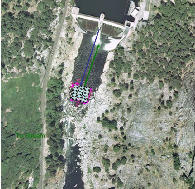
Figure 1c. Plan view of chiller location on Poe Reach; Pipe size = 4 ft; flow rate = 200 cfs
