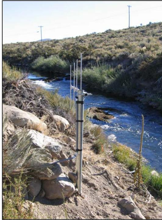
**Figure 2.** Upstream antenna location of fixed station receiver at lower end of the MGORD in September, 2005.
