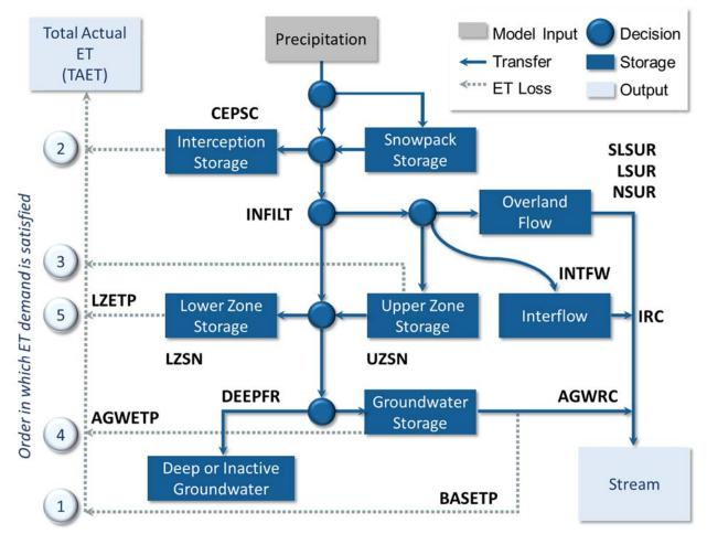
Figure 3-2. Hydrology model schematic (based on Stanford Watershed Model).
