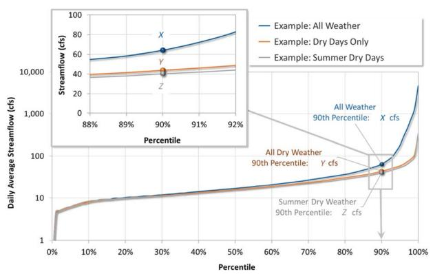
Figure 3-24. Example flow-duration curve analysis to define summer low-flow critical conditions (not based on the Shasta Basin).
