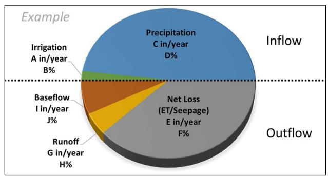
Figure 3-19. Example calibrated water balance for modeled watershed (not based on the Shasta Basin).
