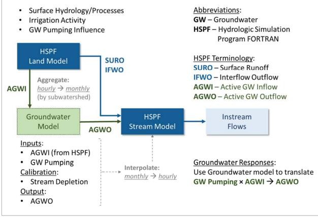
Figure 3-15. Development of groundwater response functions for LSPC using a groundwater model.
