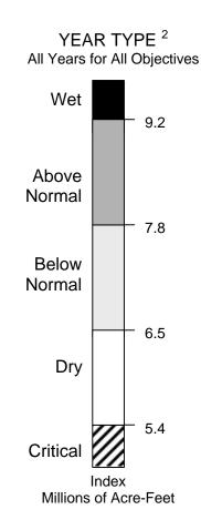
A cap of 10.0 MAF is put on the previous year's index (Z) to account for required flood control reservoir releases during wet years.
