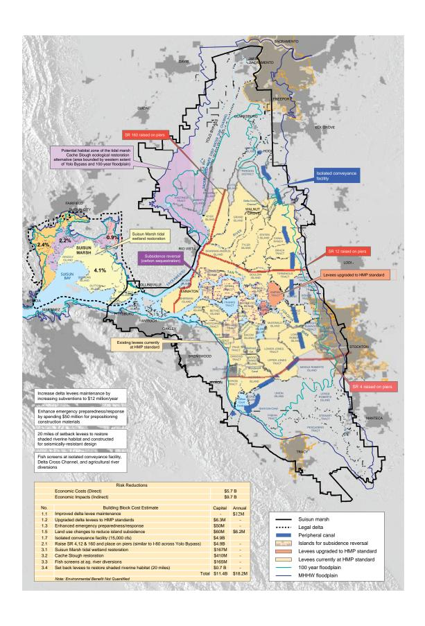
FIGURE 17. DRMS Scenario 3: Isolated Conveyance Facility
