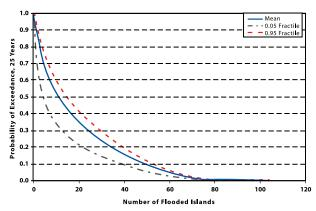
FIGURE 10. Probability In A 25 Year Exposure **Period Of A Number Of Simultaneous Levee Failures** From A Seismic Event
