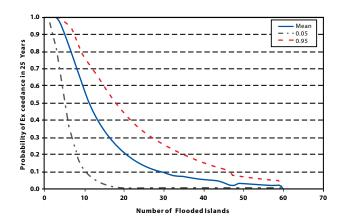
FIGURE 13. Probability In 25 Years Of Exposure For The **Indicated Number Of Simultaneous Island Failures** (Or More) From A Flood Event
