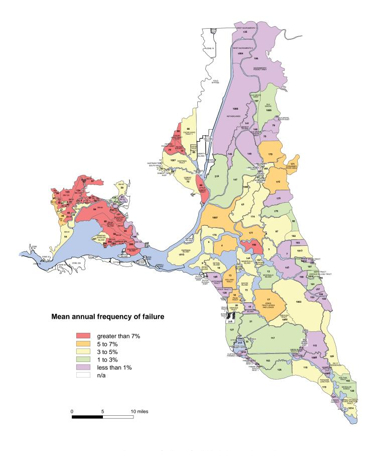
FIGURE 14. Annual Frequency Of Failures Of Individual Islands Under Flooding Events
