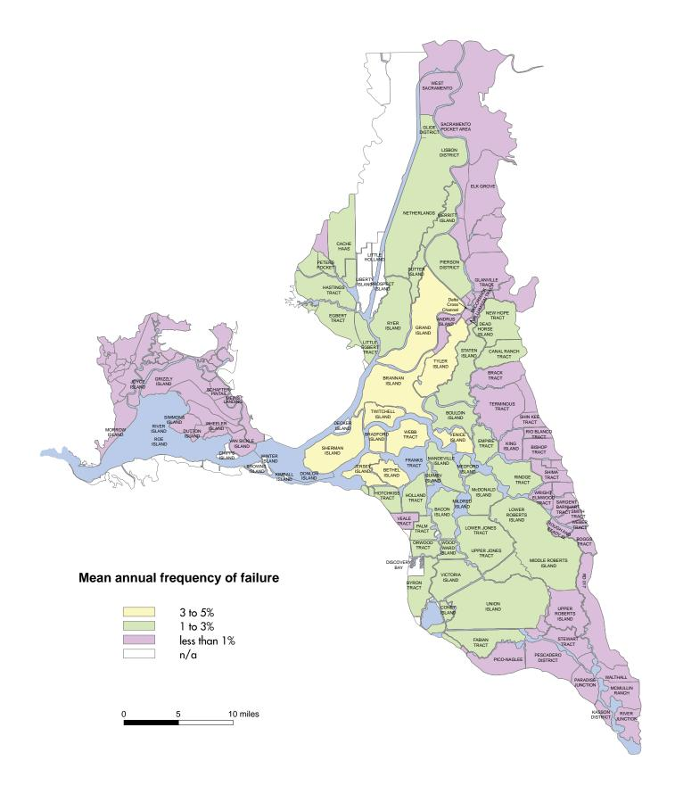
FIGURE 12. Annual Frequency Of Failure Of Individual Islands Under Seismic Events
