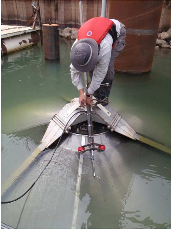
Photo 1. Mounting the velocity probe and positioning jig to the screen's cleaning system.
