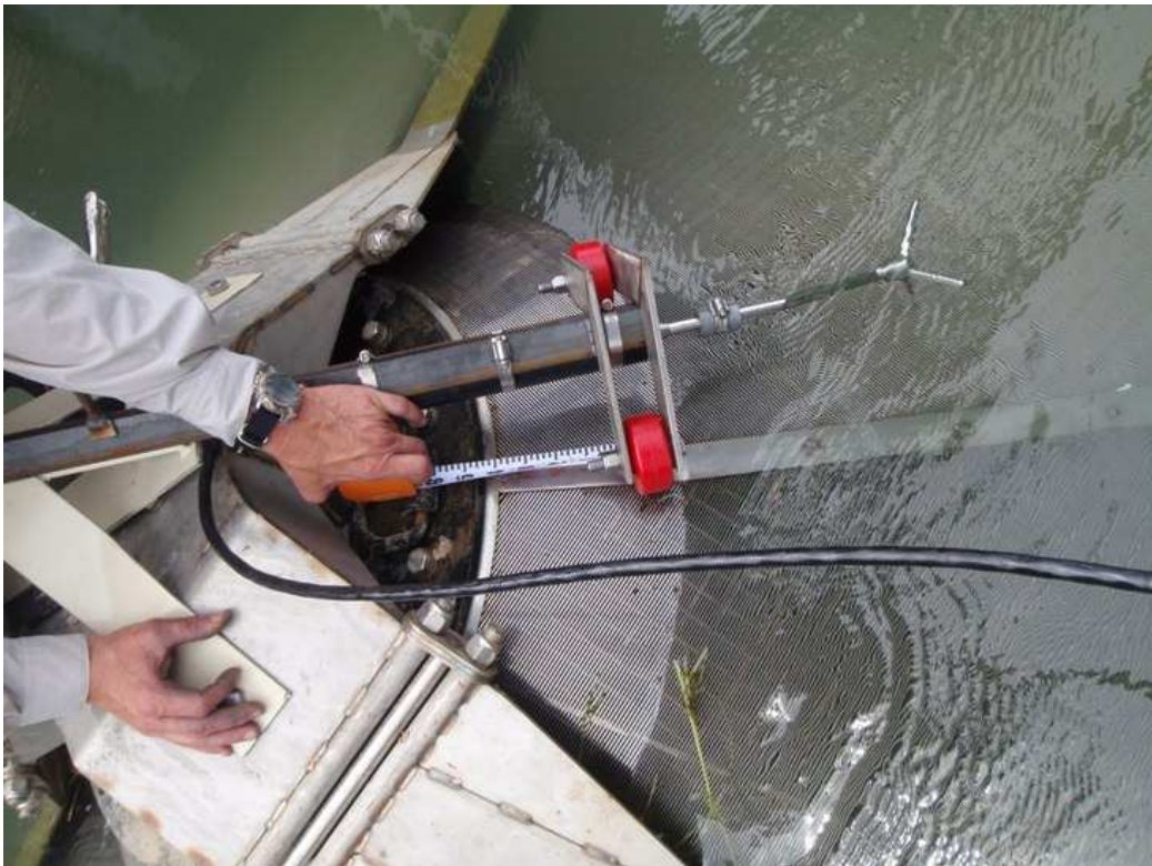
Photo 2. ADV probe in its highest position on the screen measured velocities two feet below the top of the screen panel.
