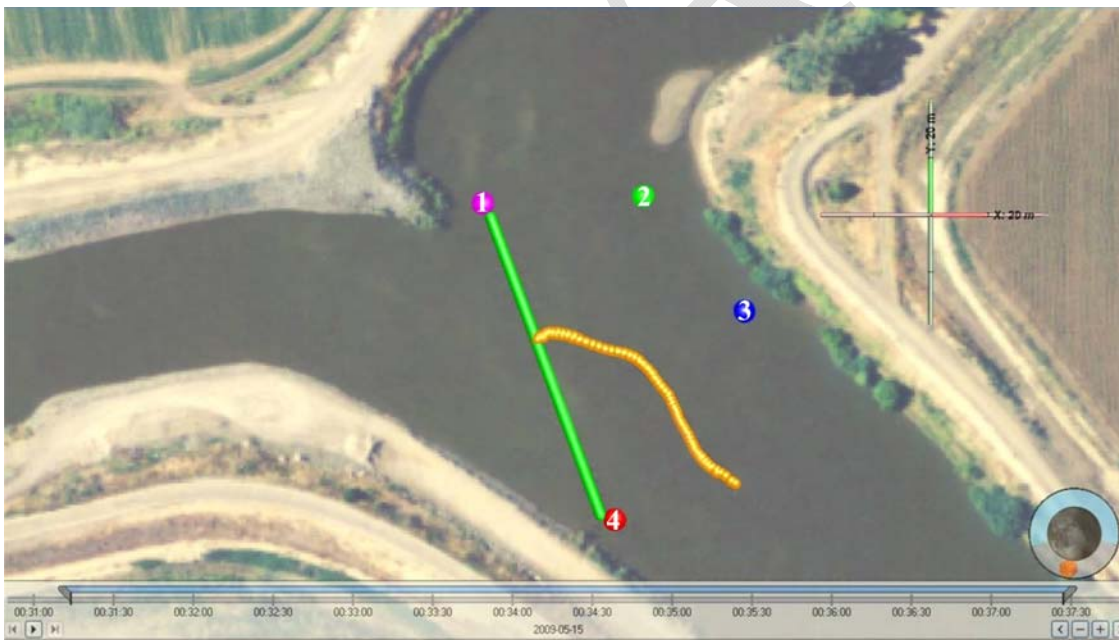
Figure 8. Tag 6514 approached the barrier in operation on 5/15/09 at 00:37 hr. The tag exhibits a smolt-like trace: downstream quickly and no predator behavior. This smolt passed through the BAFF; the 2D trace ends because hydrophone 2, 3, and 4 can't "hear" pings through the bubble curtain. This photo was taken at high tide; the green line indicates the BAFF location and the colored circles indicate the location and number of the hydrophones.
