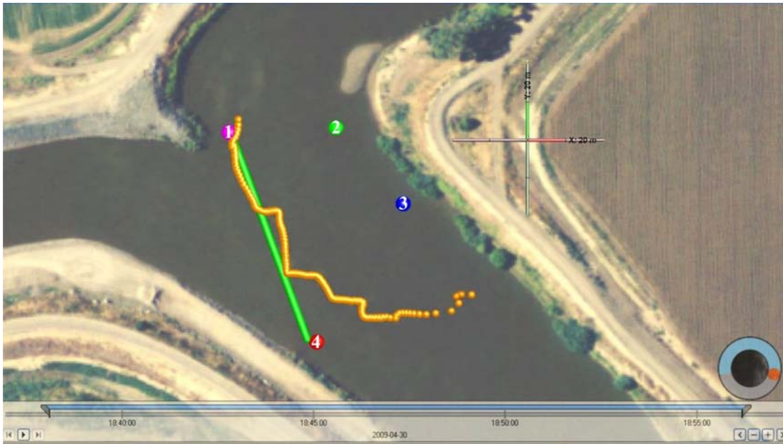
Figure 9. Tag 5344 approaches the operating BAFF on 4/30/09 at 18:46 hr. Upon this fish's first approach to the BAFF, it is deterred. This photo was taken at high tide; the green line indicates the BAFF's physical location and the colored circles indicate the location and number of the four hydrophones. With stream velocity, the bubble barrier is carried downstream of this green line.
