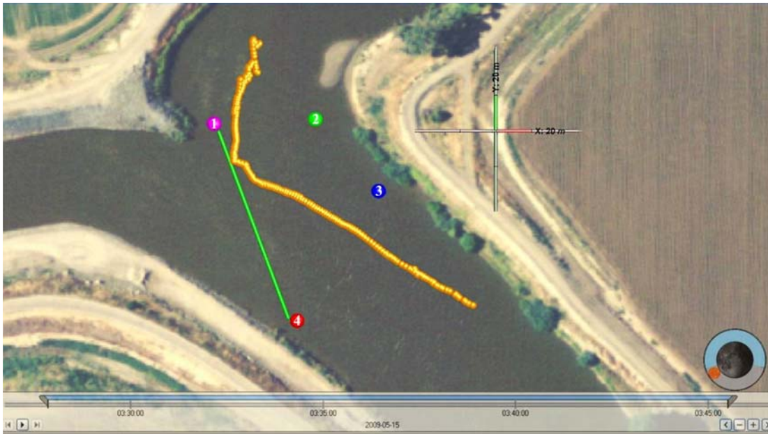
Figure 7. Tag 5674 approached the barrier in operation on 5/15/09 at 03:38 hr. The tag exhibits a smolt-like trace: downstream quickly and no predator behavior. This smolt was obviously deterred by the BAFF. This photo was taken at high tide; the green line indicates the BAFF location and the colored circles indicate the location and number of the four hydrophones.
