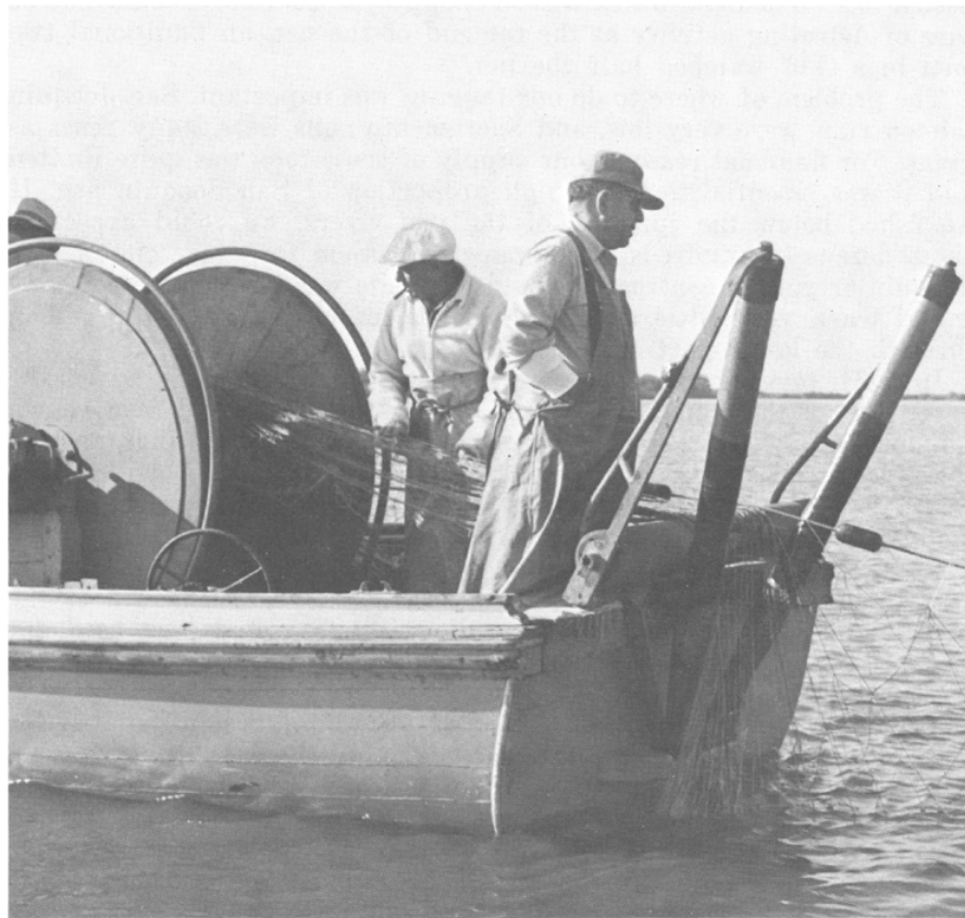
FIGURE 14. Trammel net being wound onto powered net reel on the M.V. Stripper , San Joaquin River at Prisoners Point; fall, 1965. Photograph by Richard J. Hallock.
