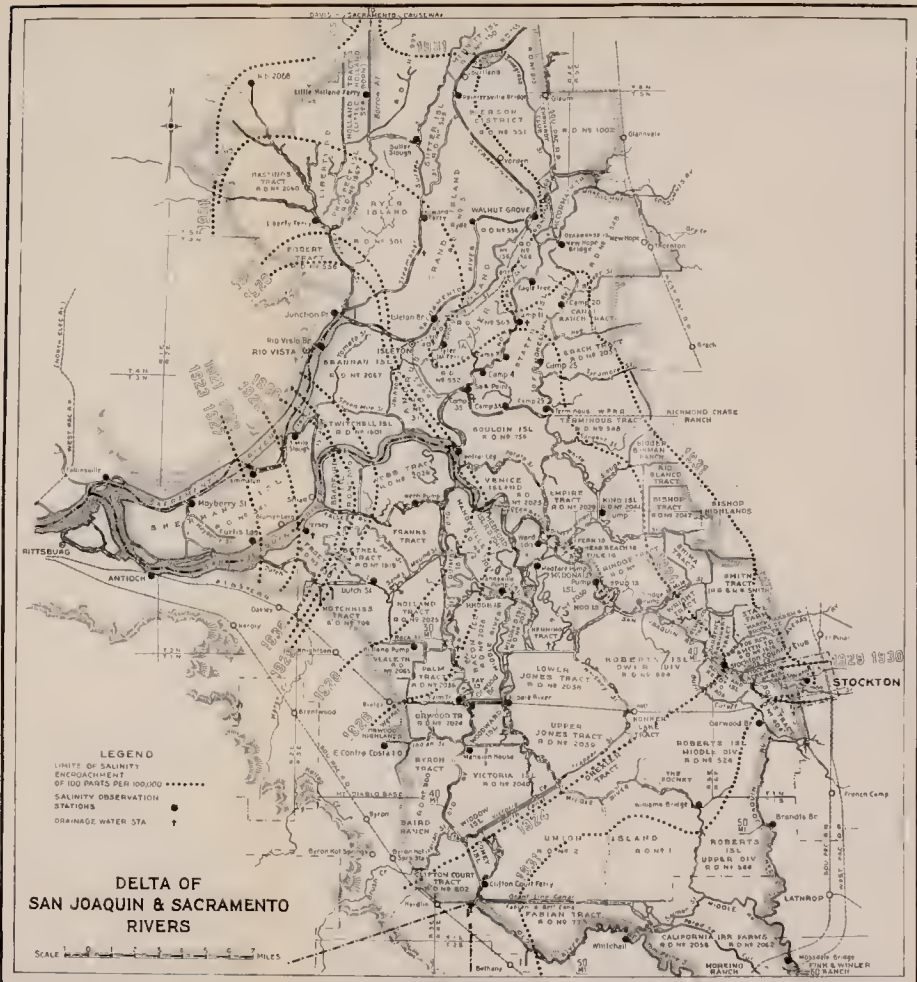
Delta of Sacramento and San Joaquin Rivers, Showing Limits of Salinity Encroachment of 100 Parts of Chlorine per 100,000 Parts of Water, 1920 to 1931, Inclusive.
