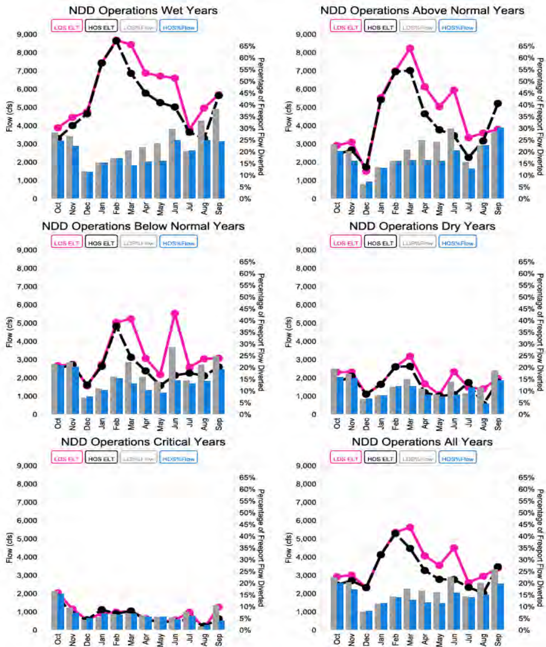
Figure 4.4. Average monthly export flows of North Delta diversion facility under HOS and LOS ELT for different year types, and percentage of total bypass channel flow exported.
