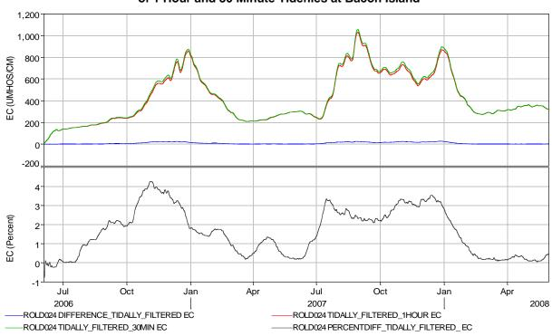
Figure 3-16 Comparison of EC Results with Time Steps of 1 Hour and 30 Minute Tidefiles at Bacon Island
