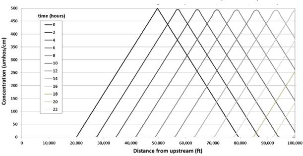
Figure 4-8 Results of DSM2-GTM for Advection in Uniform Flow along a Single Reach with Given Initial Concentration in the Middle of Reach (dx=312.5 ft)
