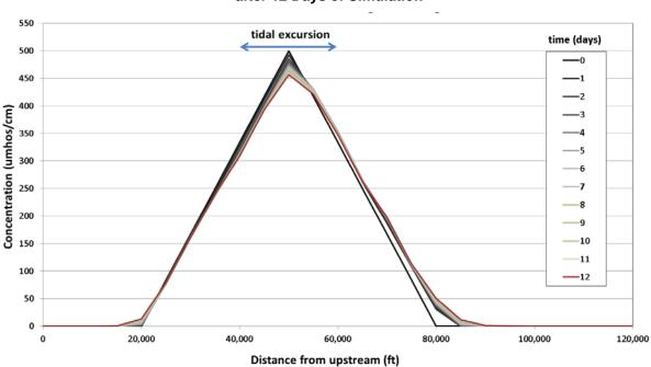
Figure 4-10 Results of DSM2-Qual for Advection in Oscillating Flow along a Reach after 12 Days of Simulation
