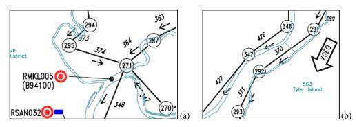
Figure 5-2 Examples of DSM2 Grid
