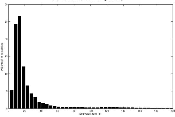
Figure 7-7 Histogram of Element Size, using Equivalent Radius (Radius of the Circle with Equal Area)
