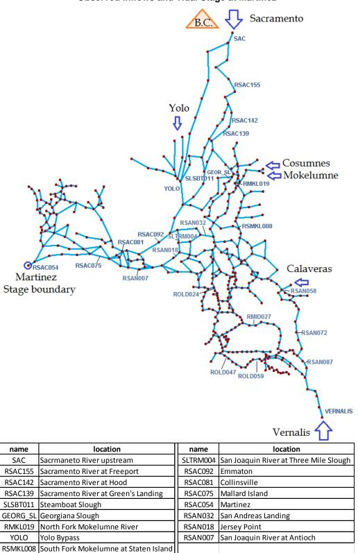
Figure 4-19 Test Case for Delta-like Grid with Observed Inflows and Tidal Stage at Martinez
