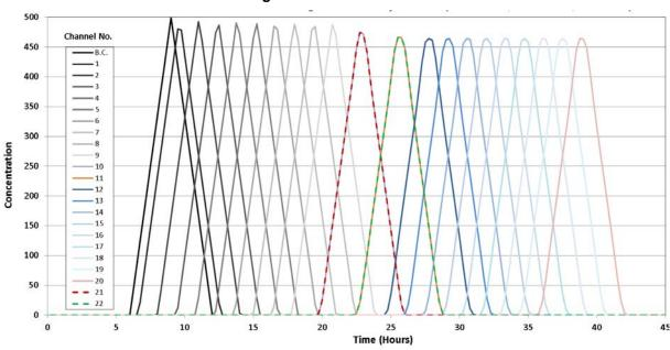
Figure 4-18 Results of DSM2-GTM for Advection in Uniform Flow along a Reach with Junctions
