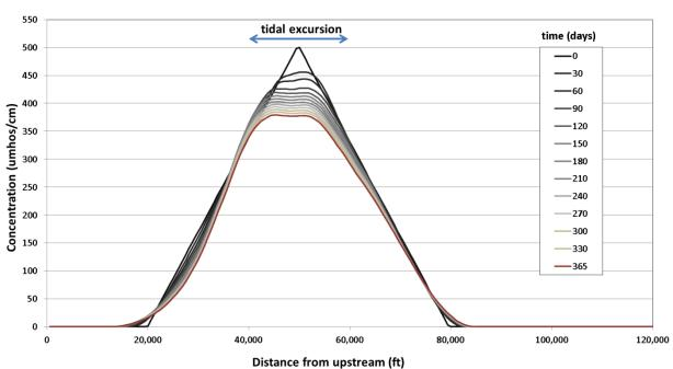
Figure 4-13 Results of DSM2-GTM for Advection in Oscillating Flow along a Reach after One Year of Simulation
