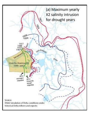
Figure 5-8 Sample Map of Maximum Salinity Intrusions of Different Drought Years Using DSM2 Simulation
