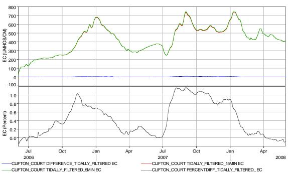
Figure 3-5 Comparison of Simulated EC with Time Steps of 15 Minutes and 5 Minutes at Clifton Court Forebay
