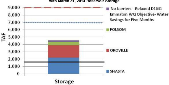
Figure 6-29 Relaxed Emmaton Objective Water Savings Plotted with March 31, 2014 Reservoir Storage
