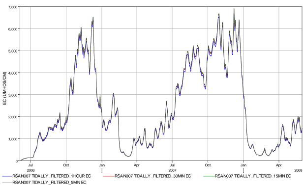
Figure 3-14 Tidefile Time Step Sensitivity at Antioch
