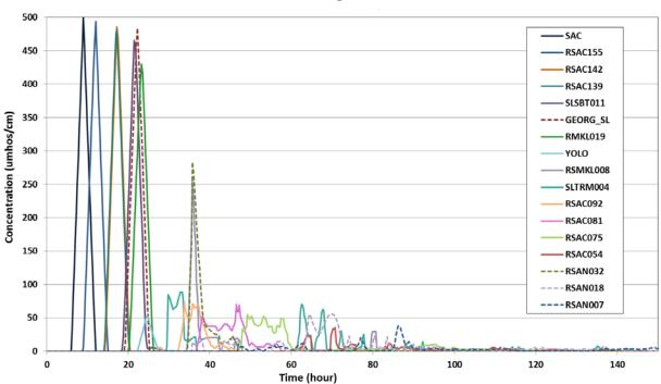
Figure 4-20 Results of DSM2-Qual for Entire Delta with Observed Inflows and Stage at Martinez
