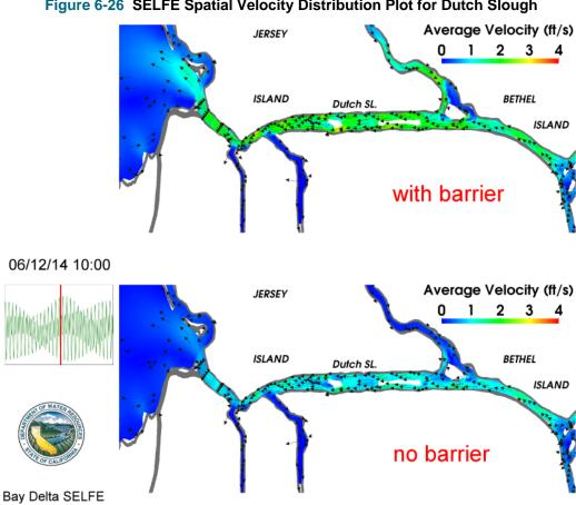
Figure 6-26 SELFE Spatial Velocity Distribution Plot for Dutch Slough
