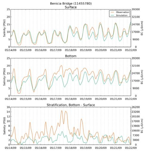
Figure 7-28 Observed Top and Bottom Salinity and Stratification at Benicia Bridge
