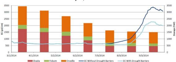
Figure 6-16 Modeled Clifton Court EC with End of Month Reservoir Storage February 20, 2014 Forecast
