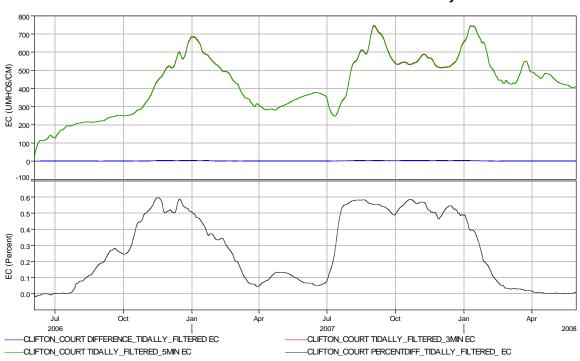
Figure 3-7 Comparison of Simulated EC with Time Steps of 5 Minutes and 3 Minutes at Clifton Court Forebay
