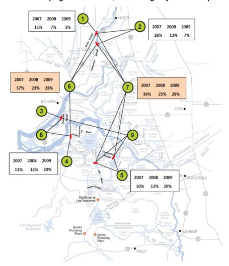
Figure 6-5 Location of Barriers and Average Electrical Conductivity Reduction at Banks Pumping Plant - Phase 2, 2009 Emergency Barriers Report
