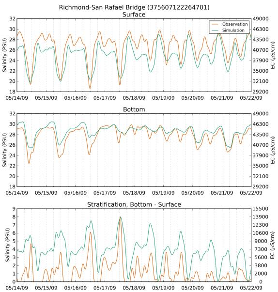
Figure 7-27 Observed Top and Bottom Salinity and Stratification at Richmond Bridge
