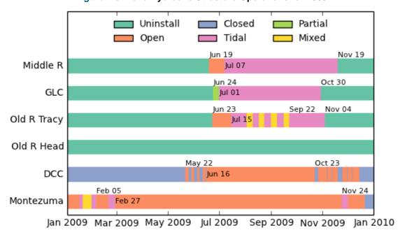
Figure 7-8 Delta Hydraulic Structure Operations for 2009
