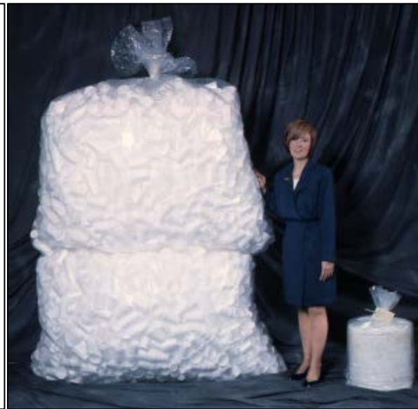
32 lbs. of foam Loose foam (left) / Densified foam (right)
