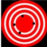
Figure 1. Demonstration of target accuracy (black marks) to a known value (bull's-eye). The figure shows very good accuracy but poor precision.
