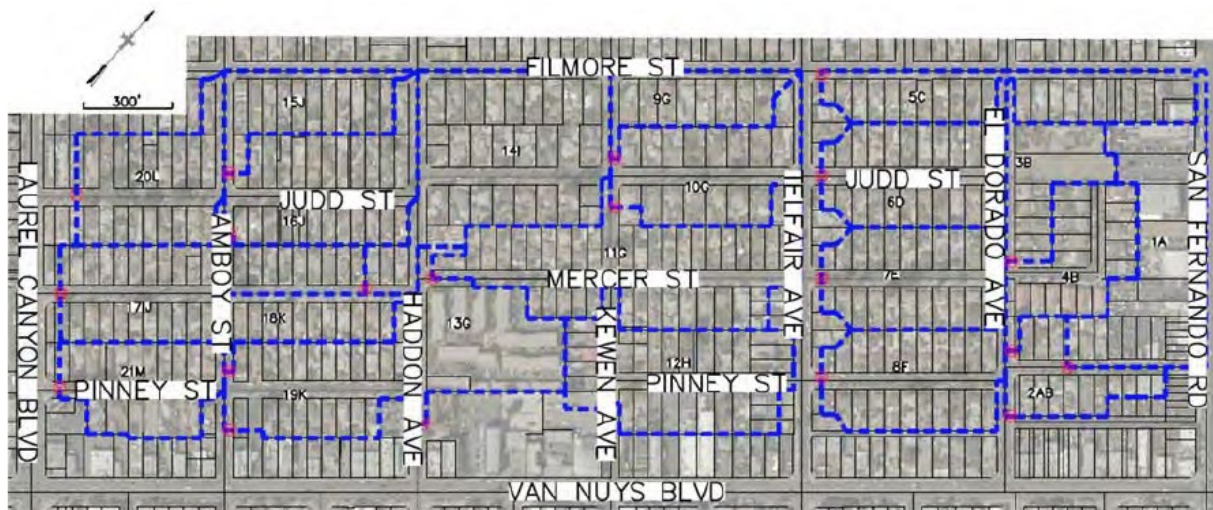
Figure B-2: LASAN Van Nuys Green Streets Drywell Project – Drainage Areas and Drywell Locations
