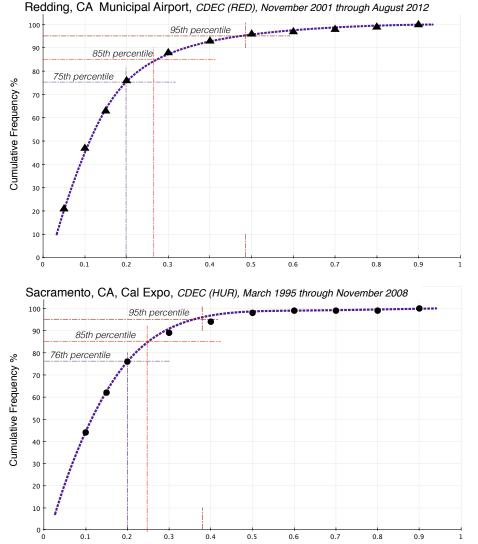
Figure 1 shows the cumulative rain depth (volume) curves for Redding, Sacramento, and Los Angeles. The weather station and the periods of record are listed on the figure. These data are based on hourly rain data reported as inches per hour. Data from days with less than 0.1 inches per day of rain are excluded.
