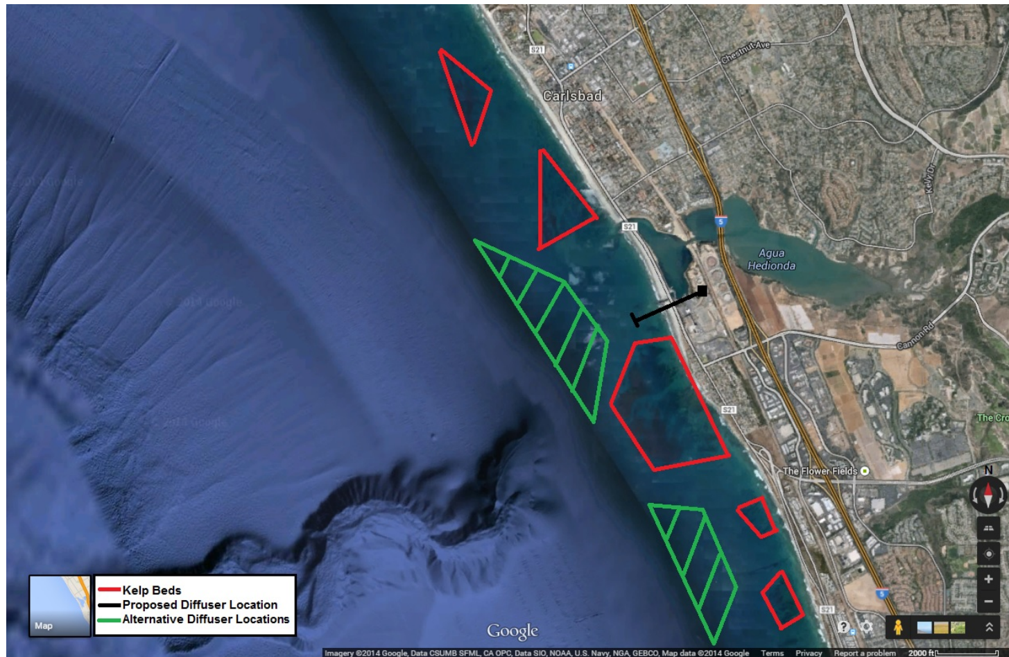
15.20-1. An aerial view of the offshore environment at the Carlsbad Desalination Project. The proposed location of the multiport diffusers is in black, the kelp beds are highlighted in red, and the green polygons are environmentally superior locations to site the diffuser array based on the location of the kelp beds alone.
