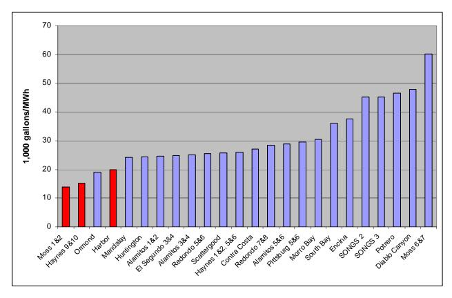
these combined-cycle units (in red) require approximately 50% less water than the average conventional fossil-fueled unit, and 67% less than the nuclear-fueled units.
