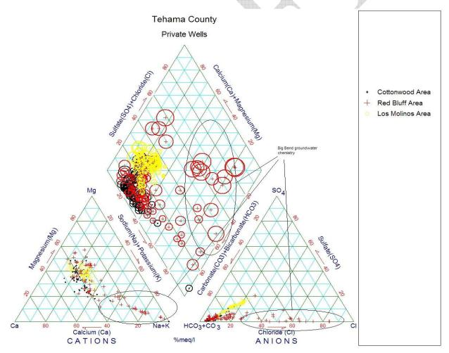
Figure 6: Piper Diagram of Groundwater Geochemical Composition
