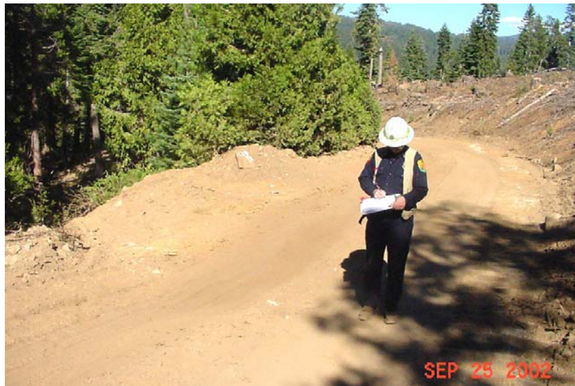
Figure 13. Pete Cafferata, CDF, recording road observations at a rolling dip. Orange box on his right hip is a hip-chain which meters-out string for tracking distances of specific road-related features along a 1000-foot sample segment.
