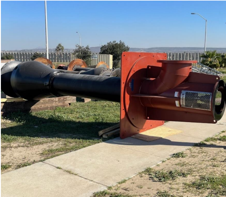
Figure 7: Closer view of one of the new influent pumps. (USIBWC 12/13/2023)
