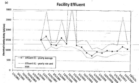
Figure 4: Historical Range of Facility Effluent Electrical Conductivity
