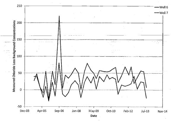
Figure 8: Well MW6 and MW7 Chloride Concentrations less Background Concentrations
