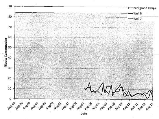
Figure 13: Well MW6 and MW7 Nitrate Concentrations Compared to Background
