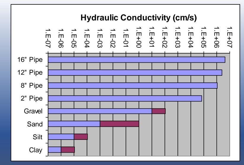
Effective hydraulic conductivities of well casings are orders of magnitude greater than layered sediments
