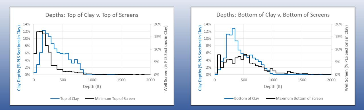
Summary of well screen depths within the extent of the Corcoran Clay from individual well completion reports. Analysis for each PLS section required to identify conduits.
