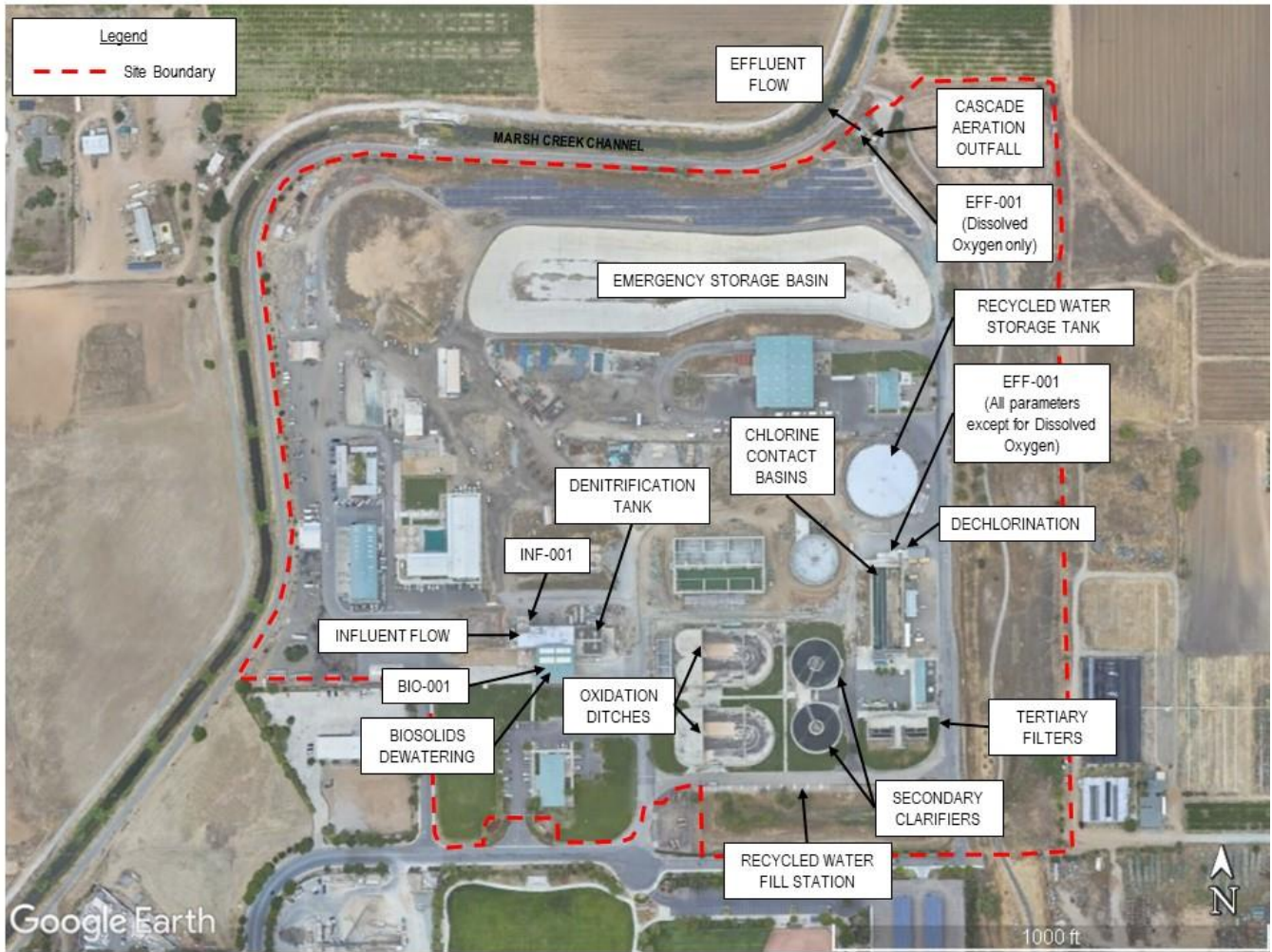
Figure B-2. Existing Facility Site Layout
